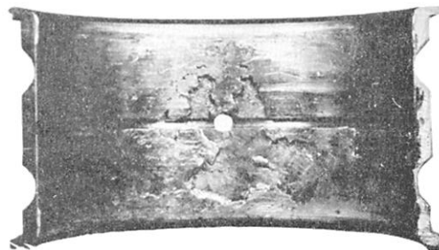
121.5 Figure 3-21.—Bearing failure resulting from wiping and excessive temperatures.
